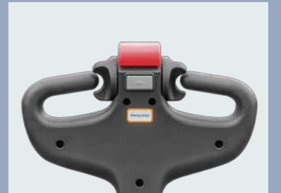
The upright-tiller running function allows it to work within confined space, such as container
